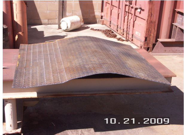
Image 14. Holding a pasteboard on edge behind each root, draw the upper root contour on the pasteboard. Then take it to a fabricator who can duplicate that contour in scrap diamondplate.
